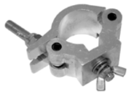
Ordercode: TOP-18 Half Coupler 500kg For D50mm Tube W50
